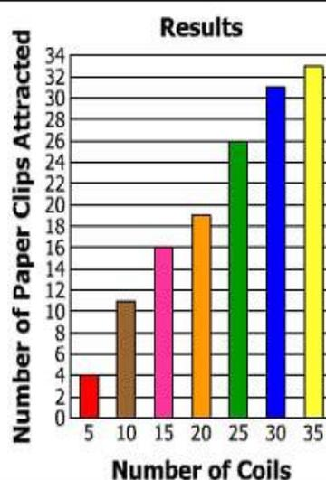
A student conducted an investigation testing the strength of an electromagnet. The dependent variable in this investigation was the —
